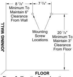
Figure 5 - Mounting Screw Locations
